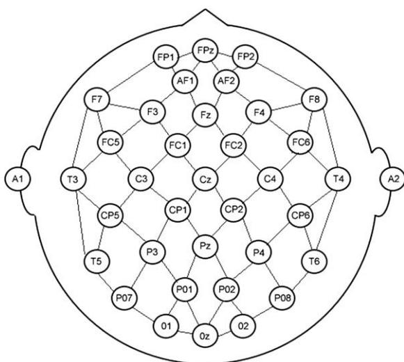
**Fig. 1.** Extended International 10–20 montage used for recording. Lines between electrodes indicate nearest-neighbor bipolar electrode pairs that were averaged for reattributed power calculations (Cook et al., 2002).
